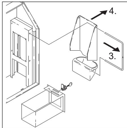
→ Use a screwdriver to lever off the angled hinge rod behind the edging of the opening and pull it out.
