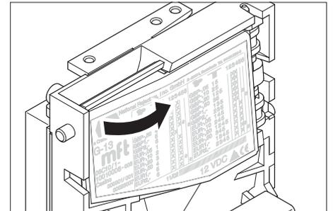
→ Open the coin acceptor, and clean the coin channel with a moist cloth and washing liquid.
