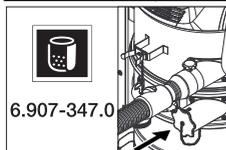
*When using the disposal bag, the lower suction nozzle must be tightly sealed.*
