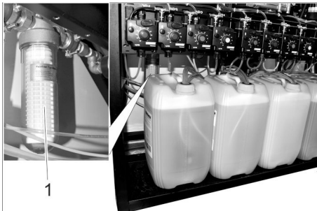
1 Filter for frost-protection pump
